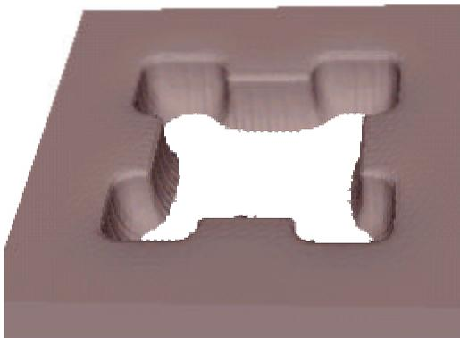
Figure 6. Three-dimensional resist profile of a  $1.0\mu\text{m}$  contact with  $0.4\mu\text{m}$  serifs in PBS.
