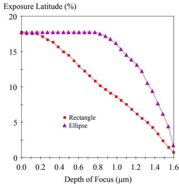
Figure 10. The process window of Figure 9 is analyzed by fitting all the maximum rectangles and all the maximum ellipses, then plotting their height (exposure latitude) versus their width (depth of focus).
