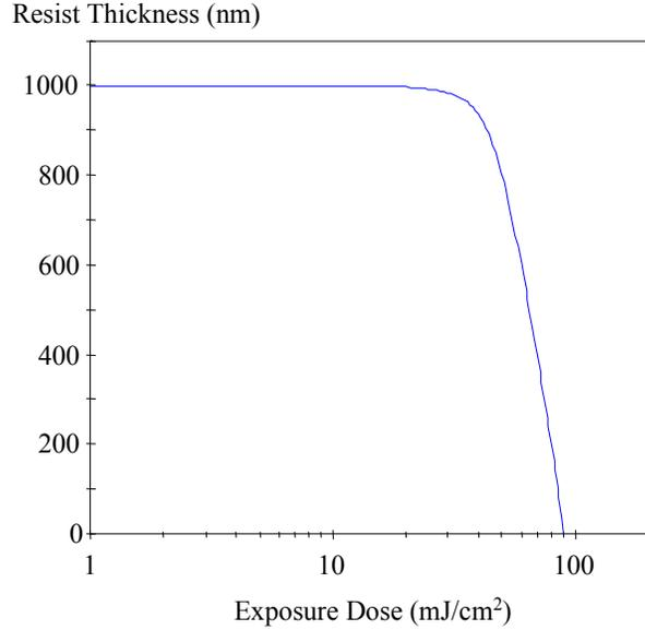
Figure 1. Typical photoresist contrast (H-D) curve for a positive photoresist.
