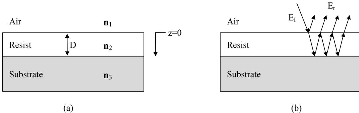
Figure 4. Film stack showing geometry for the swing curve derivation (oblique angles in (b) are shown for diagrammatical purposes only).
