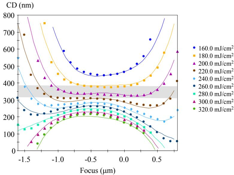
Figure 6. Example of the effect of focus and exposure on the resulting resist linewidth (symbols) and the best fit of this data (lines) to equation (23).
