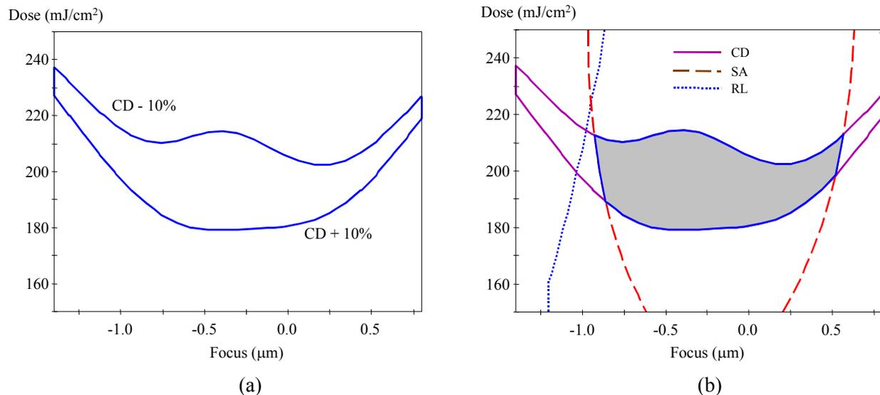
Figure 9. The focus-exposure process window is constructed from contours of the specifications for (a) linewidth, or (b) as an overlap of linewidth (CD), sidewall angle (SA), and resist loss (RL) specifications. The shaded area shows the overlap.
