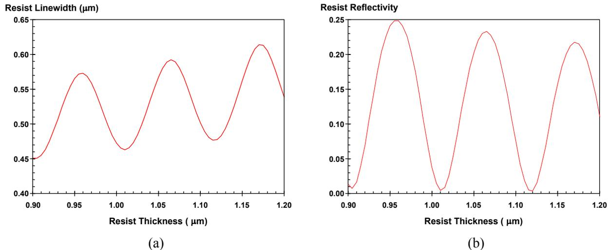
Figure 3. Swing curves showing a sinusoidal variation in (a) resist linewidth, and (b) reflectivity as a function of resist thickness.
