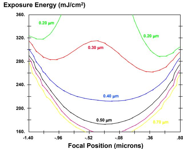
Figure 8. Displaying the fit to the data from a focus-exposure matrix in an alternate form, contours of constant CD versus focus and exposure.
