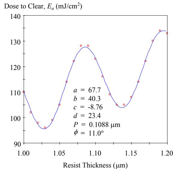
Figure 5. Best fit of equation (19) to  $E_o$  swing curve data.
