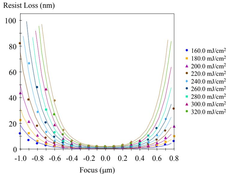
Figure 7. Example of the effect of focus and exposure on the resulting resist loss (symbols) and the best fit of this data (lines) to equation (25) for a positive resist.
