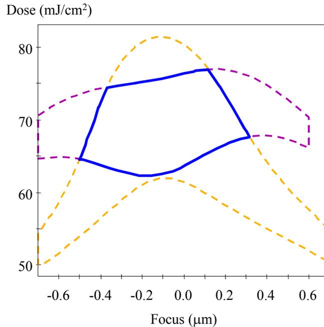
Figure 11. An example of overlapping process windows for dense and isolated lines.
