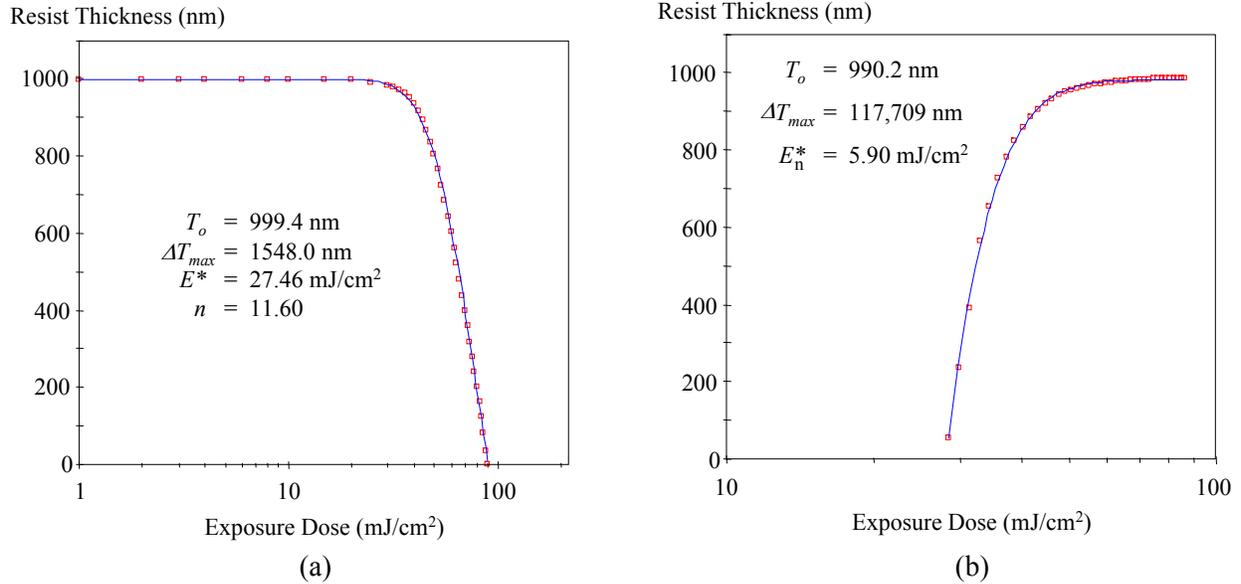
Figure 2. Examples of curve fits to contrast curve data for (a) positive, and (b) negative resists.
