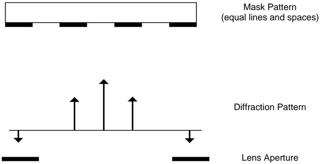
Figure 3. Typical diffraction pattern entering an objective lens aperture (assuming coherent illumination and a mask pattern of equal lines and spaces).
