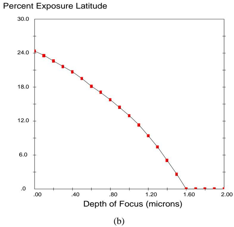
Figure 5. The process window (a) is analyzed by fitting all of the maximum rectangles, then plotting their height (exposure latitude) versus their width (depth of focus) as in (b).
